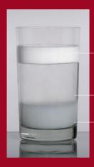
Typical behavior of Silica and waxes in water
